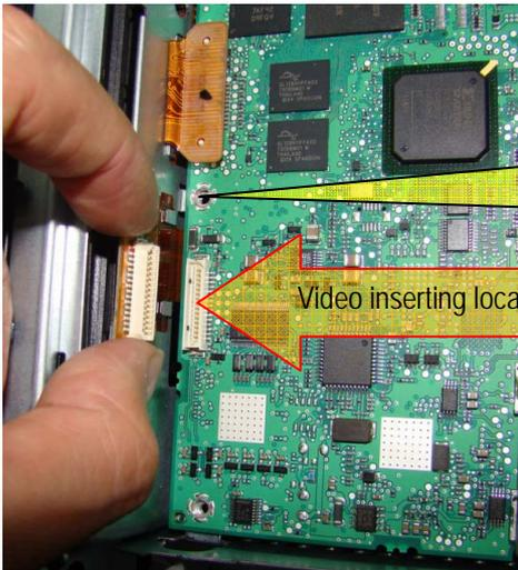
← Open the monitor by removing the top 2 screws, then the PCB is like this.
