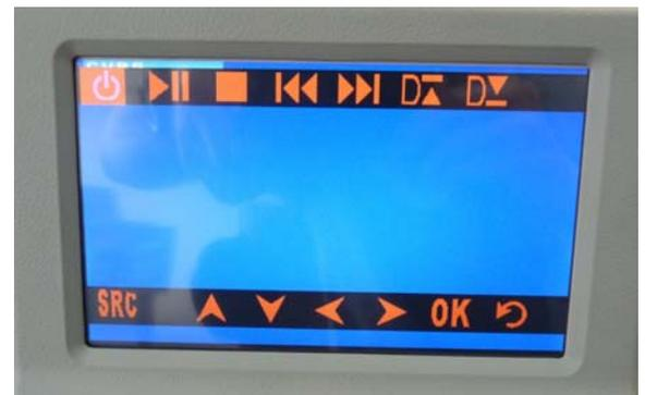
for >1 second to power off the monitor. A short press less than 1 second will make the touch screen send a 'power' command to the related video source device.
